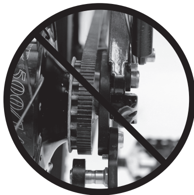
Illustration 4: Incorrect alignment of the belt
