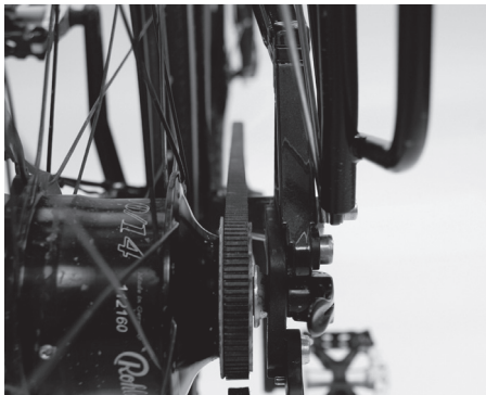
Illustration 3: Correct alignment of the belt
