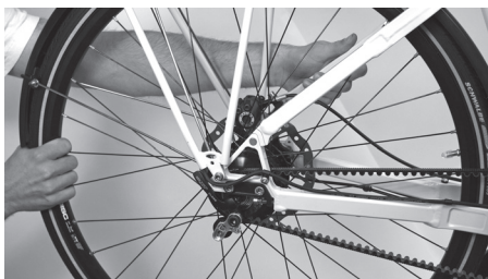
Illustration 3: Correct alignment of the belt
